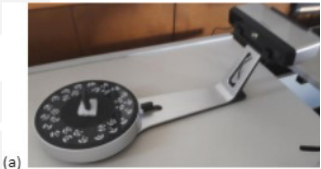
Figure 1: Overview of the scanning process with the EinScan SP desktop scanner (a). Two or more 360° scans of the flake are made (b), ensuring that the entire surface is visible in at least one scan. The mounting material is then manually removed; the two parts automatically stitched together, and a watertight mesh is fitted to the model (d).
